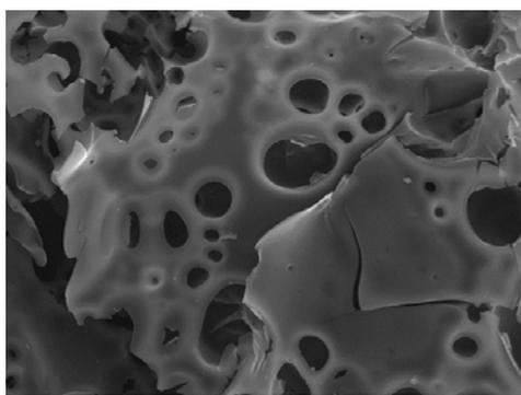
**Fig 1.** SEM images of a recently prepared in situ forming implant (ISFI-502).
